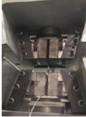
FIGURE 8. Tensile strength of rebars
